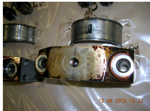
Engine Nr.3 restoration under way –cracked main bearing journal, close up.
