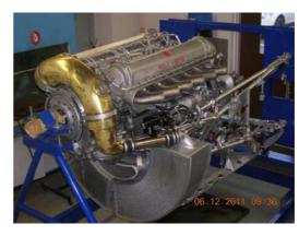
Merlin Engine Nr.2 being re-assembled in the engine shop.
