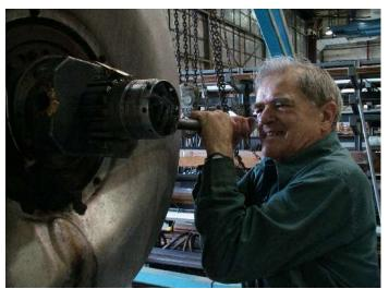
Illustration 3: Ted "Ironman"Devey checking the compression on engine no.1
