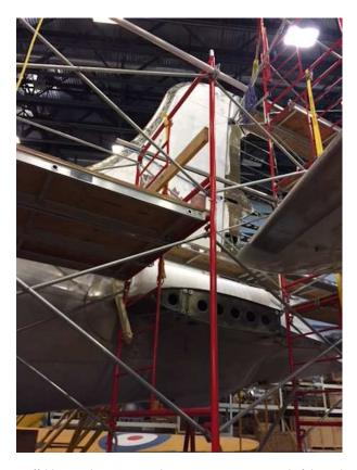
Scaffold erected next to North Star to support removal of the rudder and vertical stablizer.
