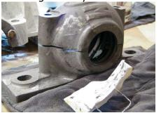
number of ties. "A lengthy wait, As part of the rehabilitation of the tripod crane (c. 1957), John has recently completed the total restoration of the pillow block casting. This required 24 hours of work.
